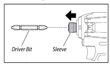
To remove the driver bit, pull the sleeve in the direction of the arrow (above) and pull the driver bit out.
