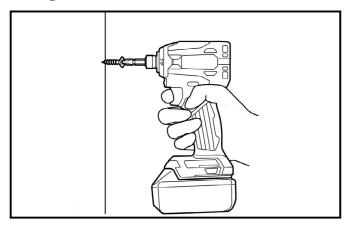
Hold the tool firmly and place the point of the driver bit in the screw head. Apply forward pressure to the tool to the extent that the bit will not slip off the screw and turn the tool on to start operation.
