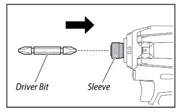
To install the driver bit, insert it into the sleeve as far as it will go (above).
